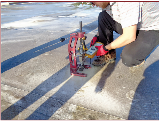
Figure 1. Pull test being performed in accordance with ANSI/SPRI FX-1 2021 version. 9
