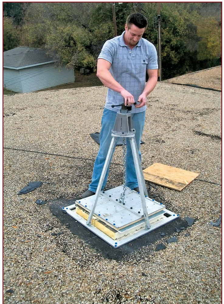
Figure 2. A worker performs a bonded test of rigid board insulation adhered to the substrate in accordance with ANSI/SPRI IA-1 2021 version. 10
