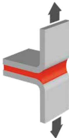
Figure 4. Example T-Peel configuration.
