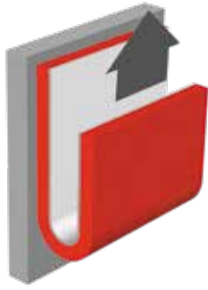
Figure 3. Typical 180-degree peel adhesion.
