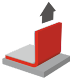
Figure 1. Typical 90-degree peel adhesion.
