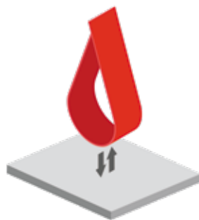
Figure 2. Loop tack measurement.
