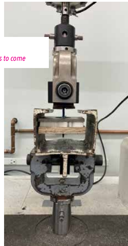
FIGURE 6. Instron tensile testing machine.
