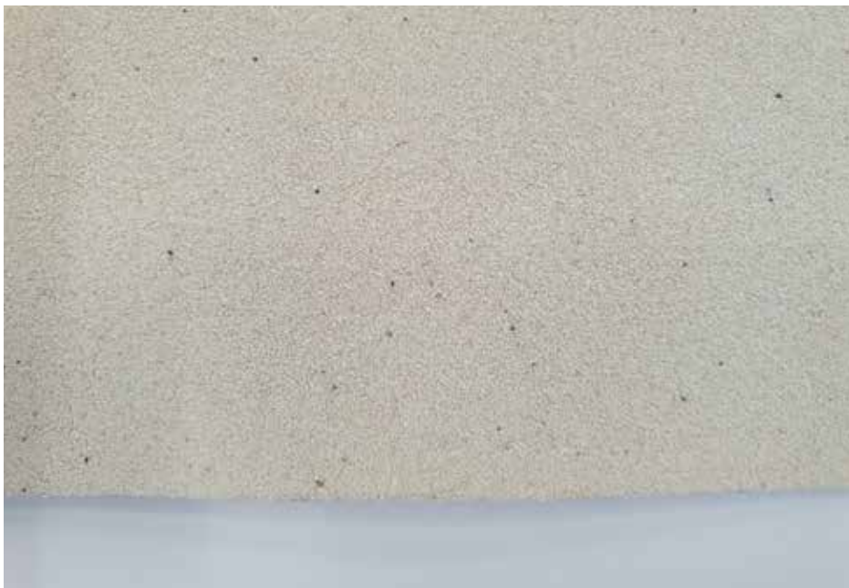
Figure 4. Bonding layer with sand granules.
