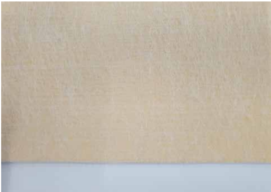
Figure 3. Nonwoven fleece bonding layer.
