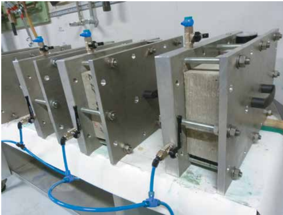
Figure 9. Apparatus used for ASTM D5385 6 testing and the study test method.
