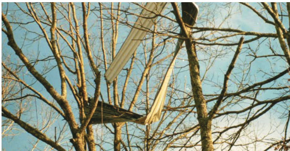
Figure 1. It is futile to worry about insulation and membrane fastening patterns when the deck itself is incapable of resisting uplift loads. Here, deck sheets had to be shaken and cut from trees after a coastal wind event.
